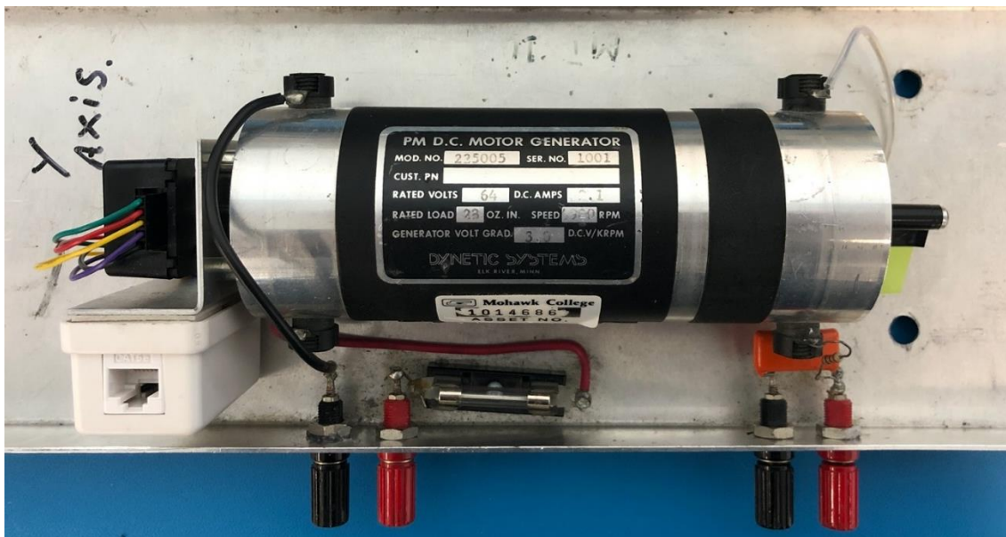
Figure 5: Permanent magnet DC motor generator used for controller testing
